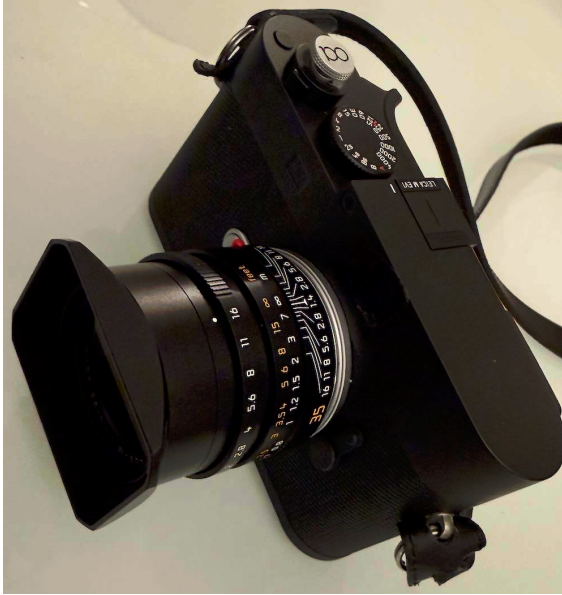
Figure 1: Leica M-EV1 (here with a thumb support, a soft release button, a carry strap, and a M-mount SUMMILUX-M 1:1.4/35 ASPH lens with UV filter (see section 41 ) and screwed lens hood).
